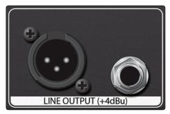
**Output.** The RC 500 provides both balanced XLR and 1/4"TRS connections. Both output connections are active all the time.
