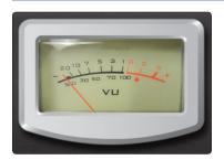
**VU Meter.** By default, the analog VU meter displays the RC 500's output level.
