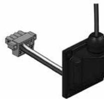
5. Use pins 1(+) and 2 (-) for connection of the loudspeaker. Use pins 3 (-) and 4 (+) for connection of additional loudspeakers in a distributed line. **Note:** Tighten pins 3 and 4 even if not used to prevent vibration of the screws.
